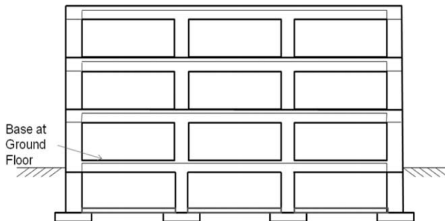
FIGURE C11-3 Base at Ground Floor Level.
